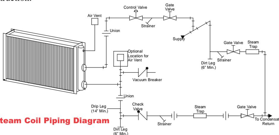
**Figure 3 - Steam Coil Piping Diagram**
