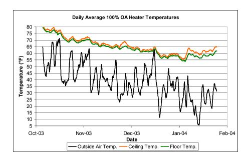
The coldest portion of the analyzed timeframe is shown in the graphs below. The first graph shows the north (re-circulating) side of the building and the second graphs shows the south (100% OA) side of the building.
