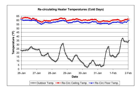
Figure 7 Coldest Days of South Side of Building Temperatures
