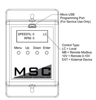
Figure 10 - MSC Front Detail View
