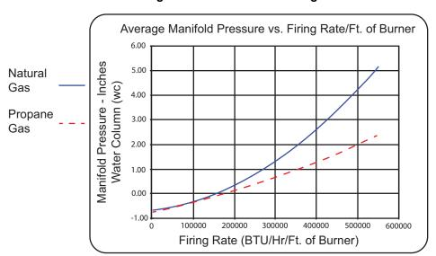
Figure 16 - Pressure vs. Firing Rate
