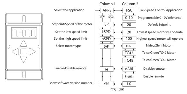
Figure 8 - RTC Speed Controller and Menu
