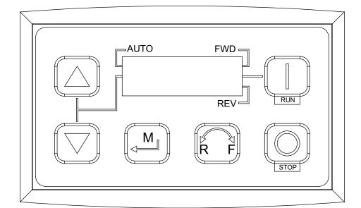
Figure 13 - VFD Screen
