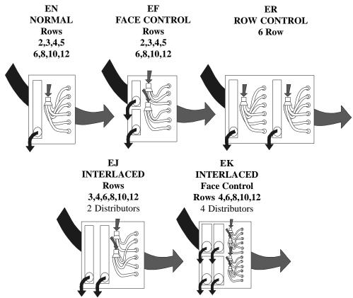
**Figure 1 - Evaporator Coils**
