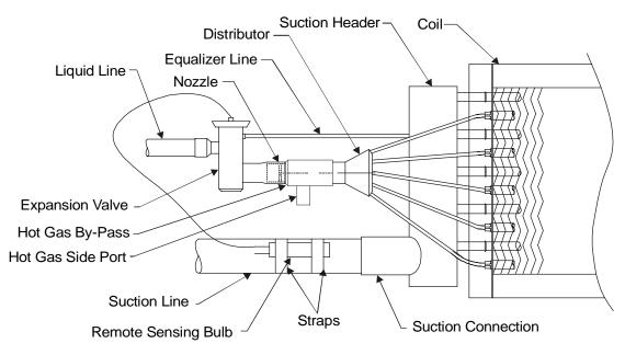
Figure 4 - Hot Gas Bypass Kit Installed
