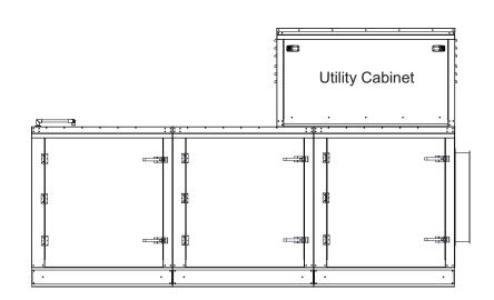
Figure 17 - Pollution Control Unit with Climate Controlled Utility Cabinet
