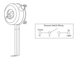
Figure 11 - Airflow Switch Installation
