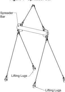
PCUs ordered with or without a KB fan all come with quantity four [4] lifting lugs factory installed on the four [4] corners of the unit. **Figure 2** illustrates a PCU with a KB fan attached.
