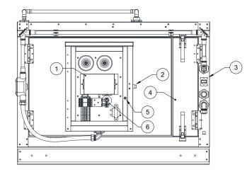
The ESP module uses one power supply per row of ESP Cells. Size 1 and 2 units will use one power supply. Size 3 through size 6 units will use two power supplies. Size 7 units will use three power supplies. The high voltage power supply contains a potentiometer. The power supply uses high voltage wire leads rated to 20K VDC. A maximum of one [1] spark per minute is allowed. If excessive sparking occurs, refer to **"Troubleshooting" on page 25**.
